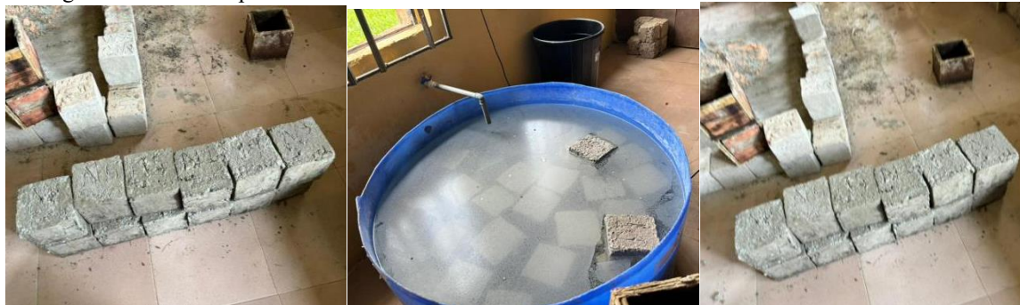
Figure 3: Cubes Cast and Cured
